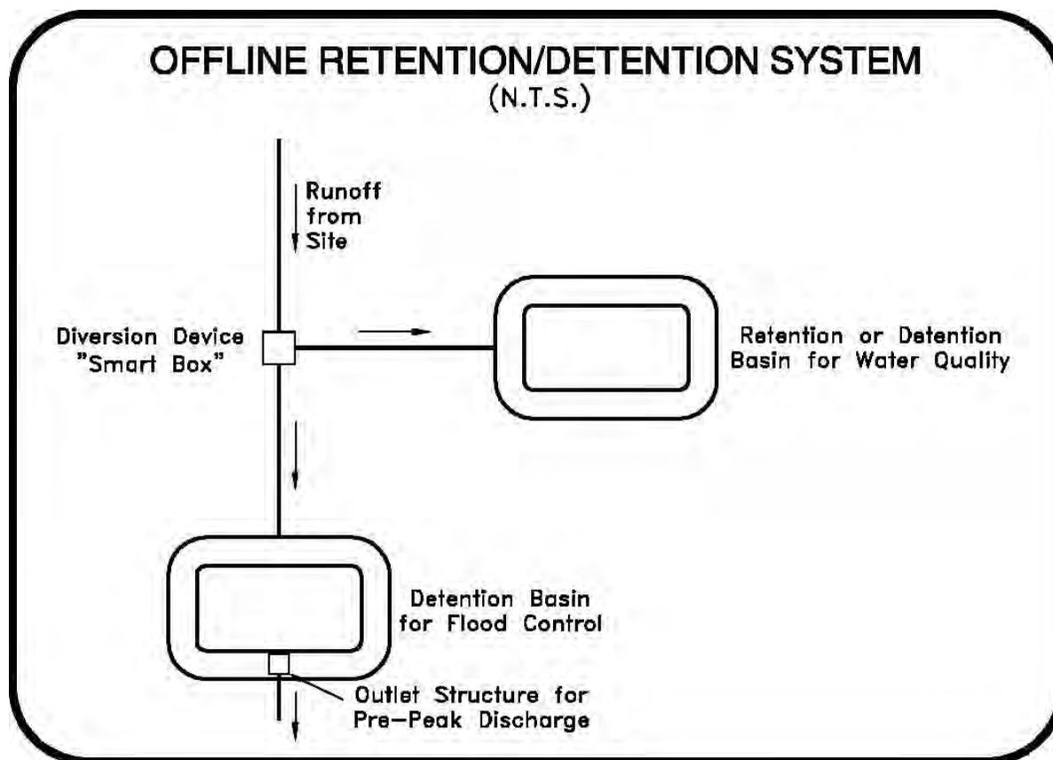
Figure 5-4. Schematic of an Off-Line Retention/Detention System.
