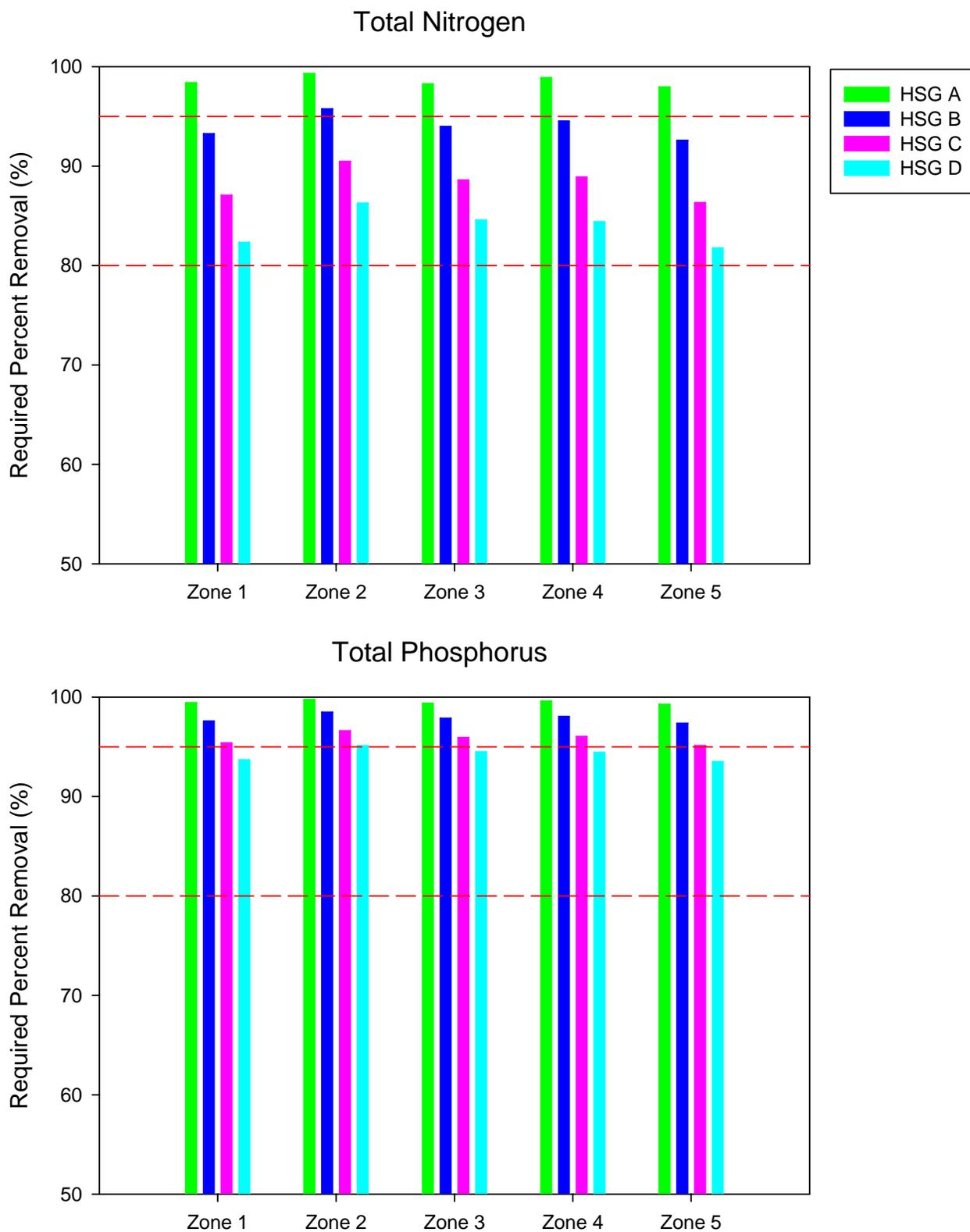
Figure 6-12. Comparison of Estimated Annual Mass Removal Efficiencies to Achieve Post-Development  $\leq$  Pre-Development Loadings of Nitrogen and Phosphorus for a Highway (75% Impervious) Development.
