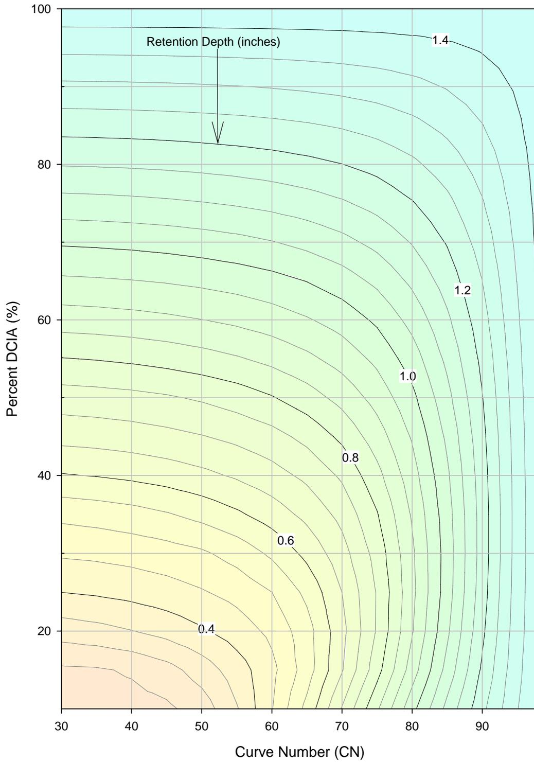
Figure 6-3. Variations in Required Dry Retention Depth to Achieve 80% Removal in the Central Zone Area (Zone 2).
