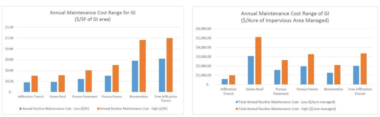
Typical annual maintenance cost-ranges for green stormwater infrastructure based on cost per square foot of green infrastructure (left) compared with maintenance costs based on square foot of impervious area managed (right). Graphs by CH2M
