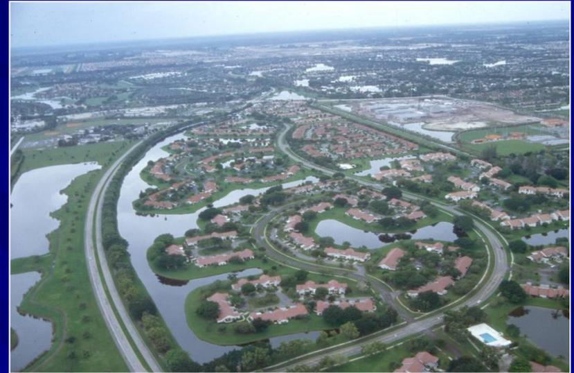
Wet Detention Lakes Can Be Integral to the Overall Development Plan
