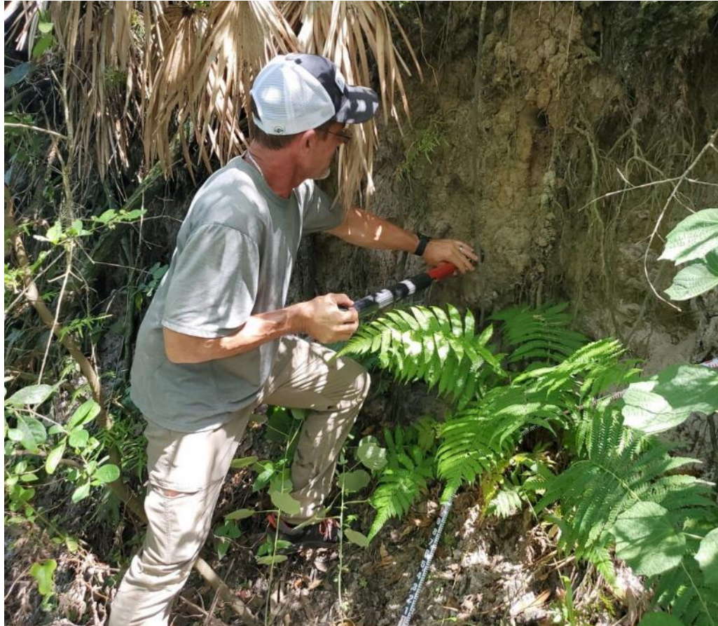
Sampling Florida bank sediments to test for phosphorus and nitrogen
