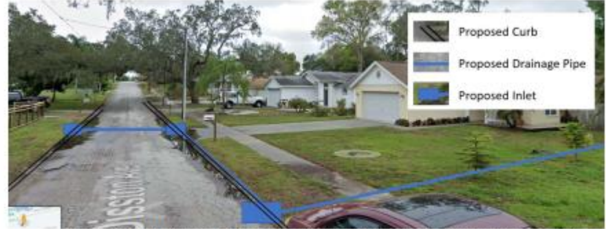
Figure 5.11 N. Disston Avenue Drainage Improvements Conceptual Layout
